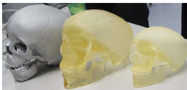
Above: A series of "printed" skulls, fabricated from layer polymer. The Objet Nanoprinter, available at the MCN allows users to transform data files into 3-Dimensional printed prototypes with a resolution of 50 microns.
